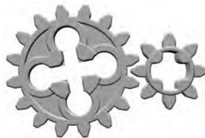
*Figure 9-17: In this example, assume that the gear on the left is the driver and the one on the right is the driven gear. This demonstrates a high gear ratio that is fast but less powerful.*
