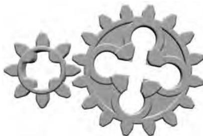
*Figure 9-16: In this example, assume that the gear on the left is the driver and the one on the right is the driven gear. This demonstrates a low gear ratio that is slow but powerful.*
