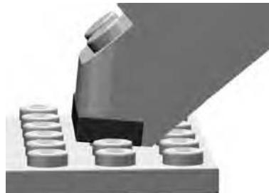
*Figure 13-15: The brick separator's unique design allows it to get close to the 1×2 plate and then lever it away from the larger plate beneath it.*
