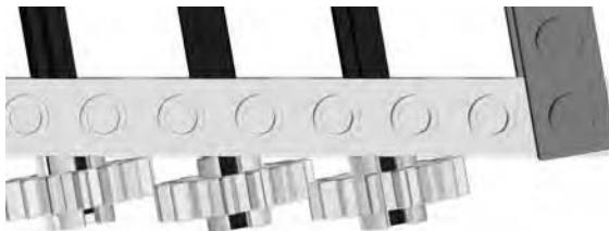
Figure 9-15: It takes only a minor misalignment to cause gears to no longer run smoothly. In the previous image, they appeared to be lined up, but in this top view, you can see that they clearly are not.
